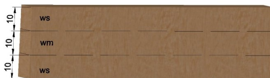
Figure 3 Moisture gradient sample ( w_m – moisture content of middle layer, w_s – moisture content of surface layer)
