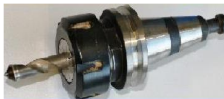
Fig. 4. Drilling bit Leitz clamped in grip.
