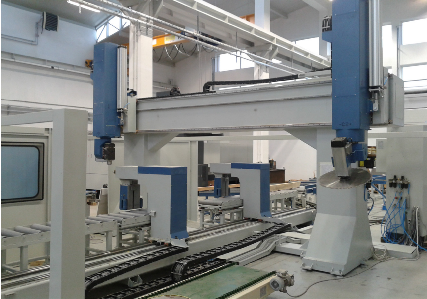
Fig.5. View of downtown carpenter "KAPPA": portal, spindles, trucks mobile systems and for discharge
