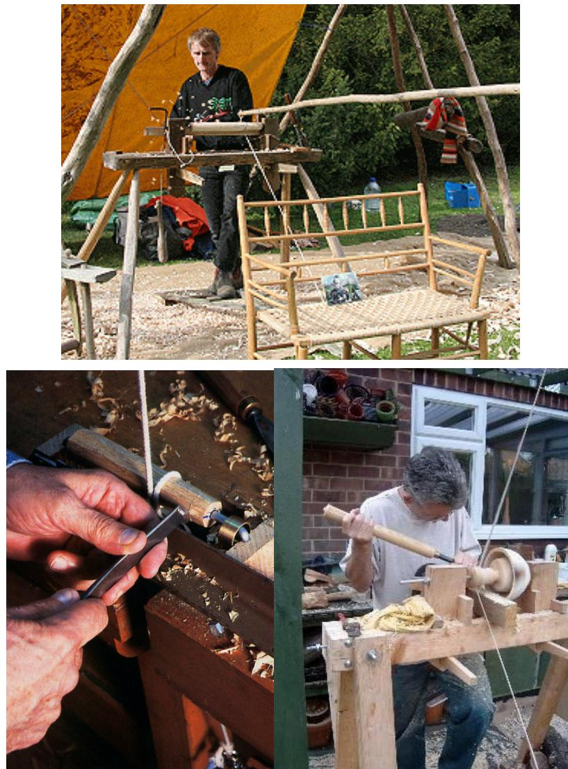
Fig.13-15. The spring pole lathe turners
