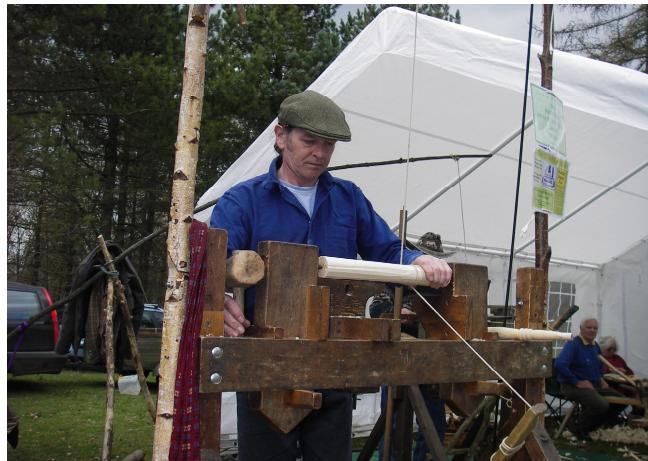
Fig.16. Association of Pole lathe Turners turning at Wendover Woods
