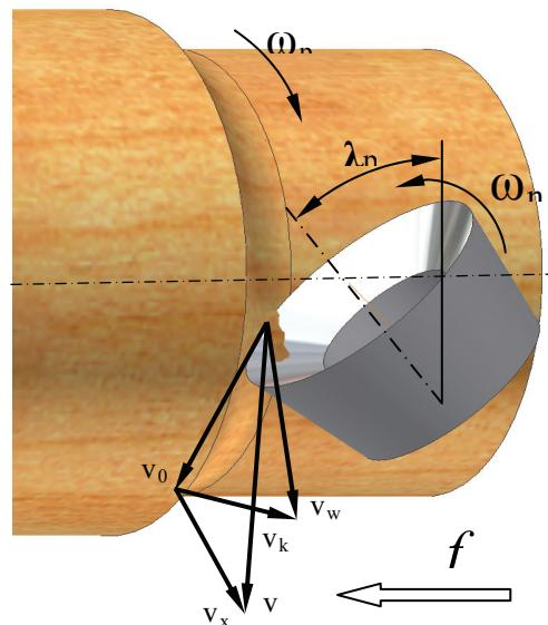
Fig.2. Kinematic dependences during machining with self-propelling disc tool.
