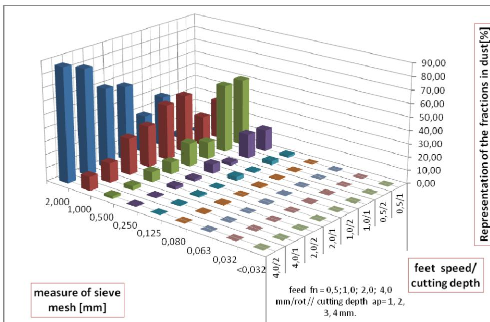
Fig. 6. The granulometric share of chips and dust of oak wood obtained during turning with SPRT at different feed speeds and cutting depth.
