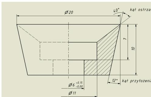
Fig.4. Parameters of cutting edge of SPRT used for research.
