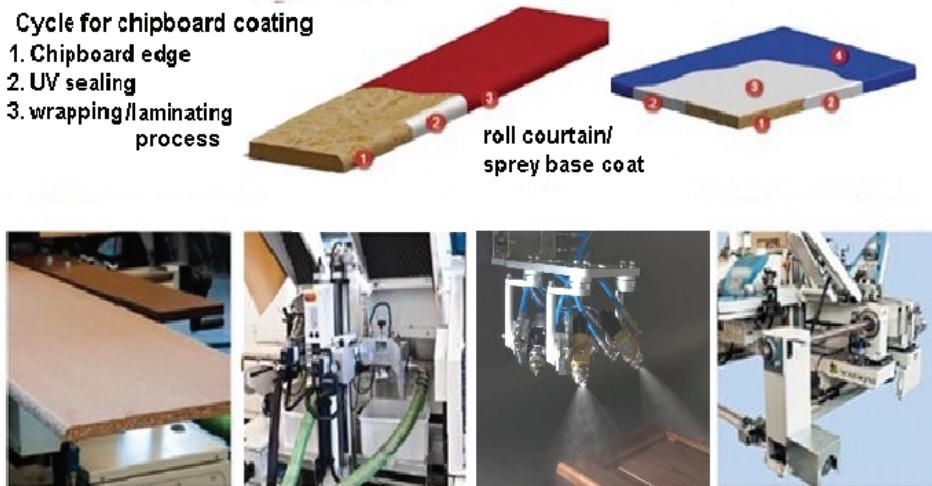
Fig. 5. Cycle for chipboard coating
