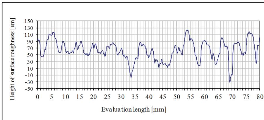
Fig.9. Profilogram of edge surface of particle board non laquered
