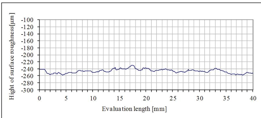
Fig.10. Profilogram of edge surface of MDF board lacquered by GEMINI equipment
