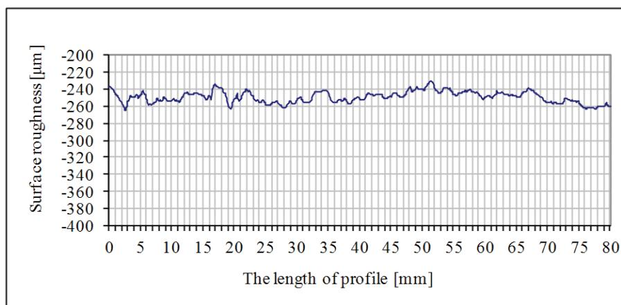
Fig. 8. Prophilogram of edge surface of particle board laquered by GEMINI equipment
