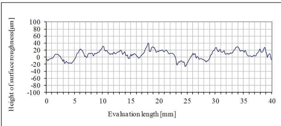
Fig.11. Profilogram of edge surface of MDF board non lacquered
