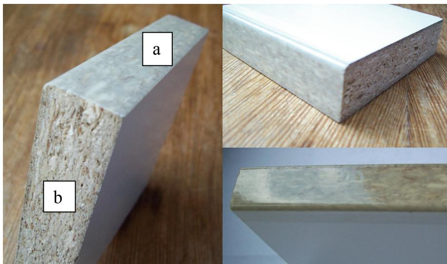
Fig. 7 . Particle board with one edge lacquered with colourless lacquer.
