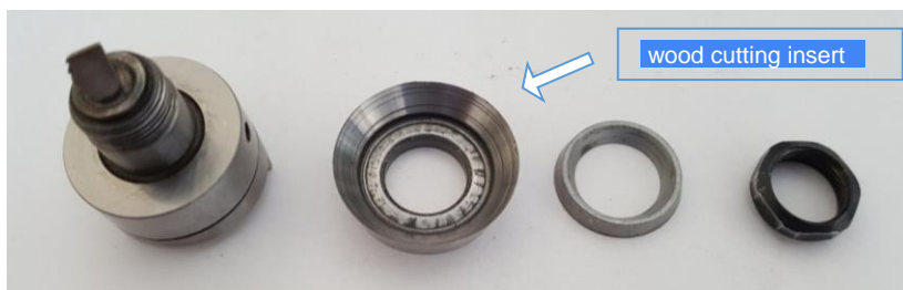
Fig.6. Construction of self-rotating SPRT tool blades
