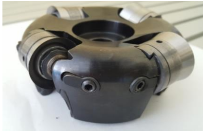
Fig.3. Standard milling head based on self-rotating blades
