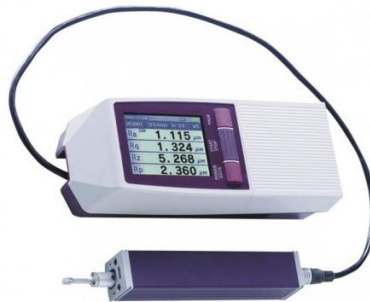
Figure 2. Profilometer, model Surftest SJ-210 – general view
