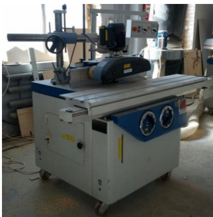
Figure 1. Woodworking spindle moulder machine, type T1002S – general view
