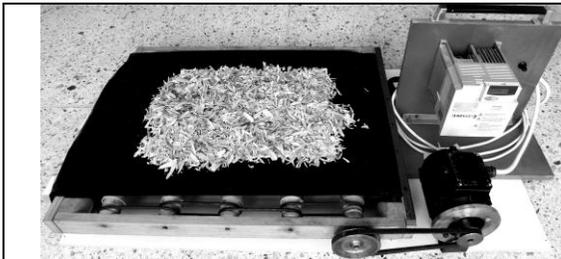
Fig. 2 Laboratory test stand for determining the angle of repose of chipped wood in a calm state and under conditions of dynamic shaking effects
