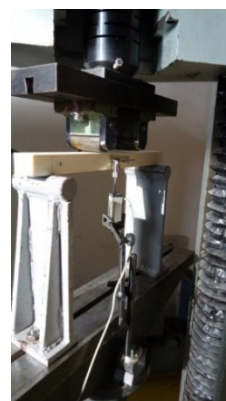
Fig. 3 Bending test, measuring deformation
