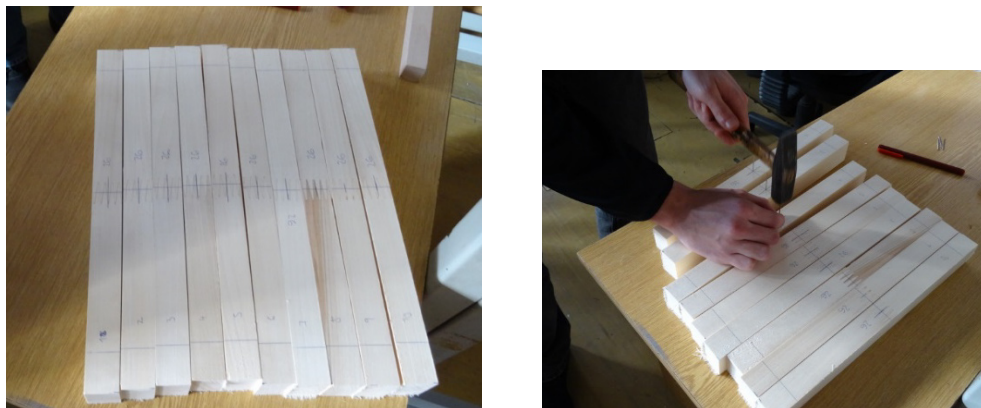
Fig.2 Sample preparation the bending test
