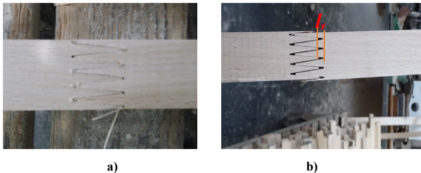
Fig. 6 Finger joint a) high quality, b) insufficient
