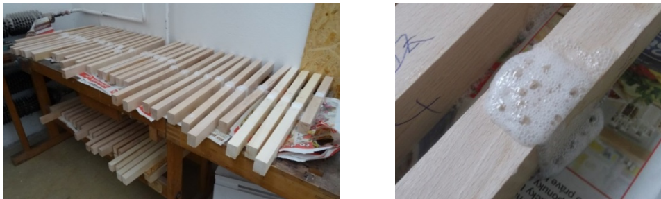
Fig. 7 Glued samples hardening with foamed up glue
