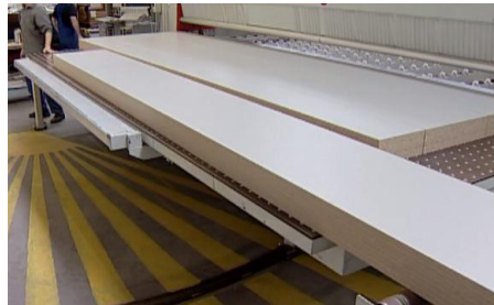
Figure 2 Cutting of board elements into strips on a panel sawing machine
