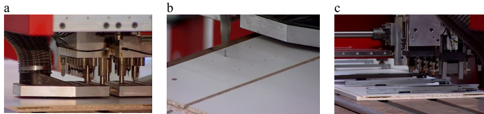
Figure 15 Execution of operations associated with the purpose and construction assembly a - hole drilling for dowels and guides, b - dowel mounting, c - guide mounting
