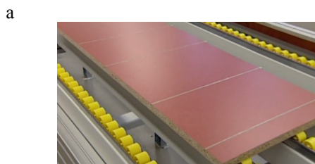
Figure 8 Panel with glued grooves; a – general view, b – single groove
