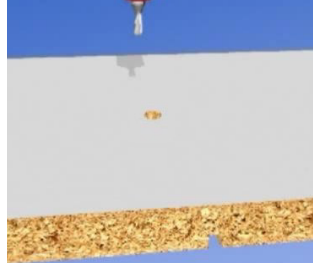
Figure 5 Drilling of the hole through the board panel allowing glue administration to the groove area
