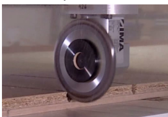
Figure 11 Execution of deep grooves
