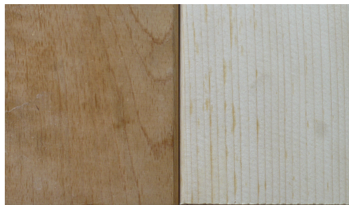
Figure 1 Spruce samples; at left thermally modified wood; at right natural spruce
