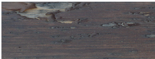
Figure 2 Destruction of coating and wood on sample HTSrR-2 after 2 years
