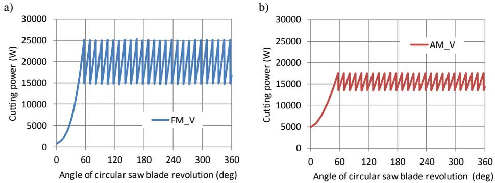
**Figure 3.** Comparison of predictions of cutting powers obtained with the use of a new developed cutting model FM\_V (a) and the Axelsson's model AM\_V (b) in the case of dry pine sawing with one circular saw blade (at the depth of cut  $H_p = 80$  mm, feed speed  $v_f = 153$  m·min<sup>-1</sup>, )
