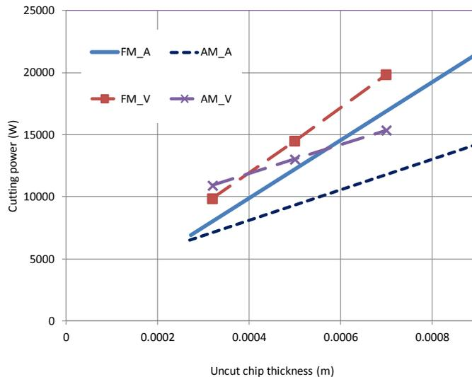
**Figure 4.** Comparison of predictions of cutting powers obtained with the use of: FM\_V model and AM\_V (for  $h = 0.00032$  m,  $0.0005$  m,  $0.0007$  m), and the models FM\_A and AM\_A in which calculations were done for the mean uncut chip thicknesses (for  $h = 0.000273\text{--}0.000913$  m) in the case of dry pine sawing with one circular saw blade
