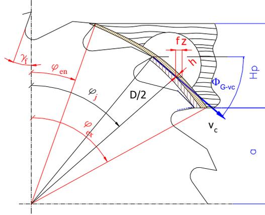
**Figure 1.** Sawing kinematics on circular sawing machine:  $H_p$  workpiece height (depth of cut),  $a$  position of the workpiece,  $\varphi_j$  angular tooth position,  $\Phi_{G-vc}$  an angle between grains and the cutting speed direction (Orlowski and Ochrymiuk 2013)
