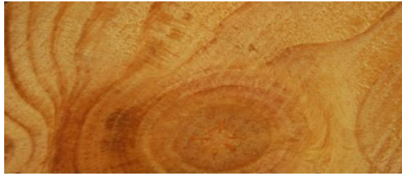
Fig. 6. Example of the cross section of pine wood sample from the Region B with an irregular annual growth
