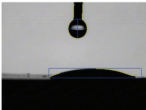
Figure 1. Determination of contact angle for poly(vinyl acetate) glue
