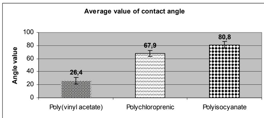
Figure 7. Measurements results of contact angle for all glues
