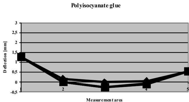
Figure 6. Graph of deflections of wood-based panel veneered with polyisocyanate glue [Oleńska et al, 2011]
