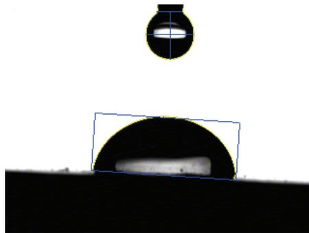
Figure 3. Determination of contact angle for polychloroprenic glue
