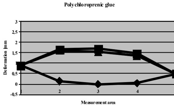
Figure 4. Graph of deflections of wood-based panel veneered with polychloroprenic glue [Oleńska et al., 2010]
