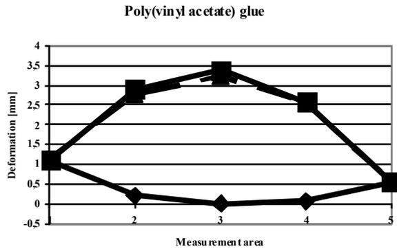
Figure 2. Graph of deflection of wood-based panel veneered with poly(vinyl acetate) glue [Oleńska et al., 2010]
