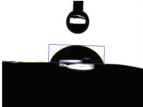
Figure 5. Determination of contact angle for polyisocyanate glue
