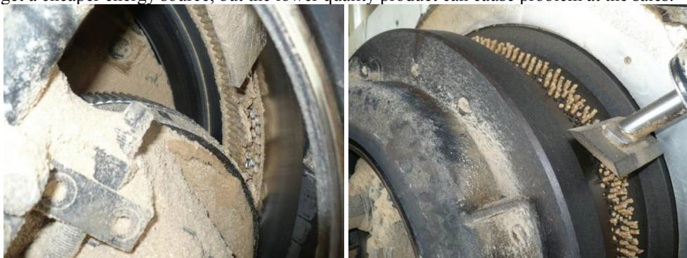
*Figure 1. Master unit of the pelleting equipment: ring die and roller shells*
