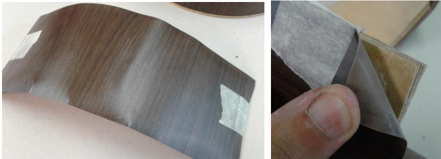
Figure 2. 1 - Test samples with poor adhesion between the PVC foil and the substrate; 2 – No adhesion can be seen by the ends of the samples, of the fact that the glue dries too fast by the initial vacuum
