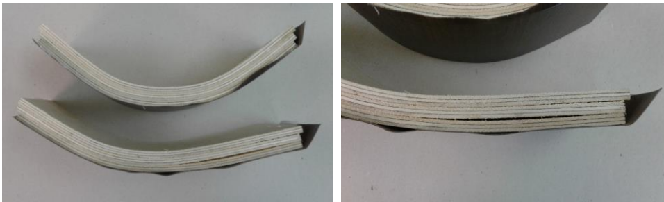
Figure 3. 1 - Self debonding of the test samples
