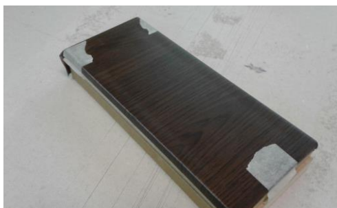
Figure 5. Uneven surface of the foil with bubbles in the end of the sample, by the high amount of the adhesive
