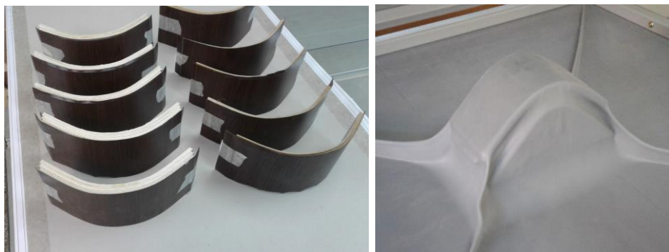
Figure 1. 1 - Test samples series; 2 - Test sample vacuumed under the rubber membrane and the matrix of bending with 100 mm radius of curvature
