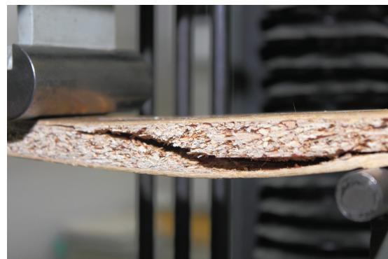
Fig. 5. The damage of the panel with bamboo stripes
