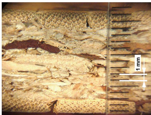
Fig. 6. The longitudinal cracks of bamboo stripes (top of the picture)
