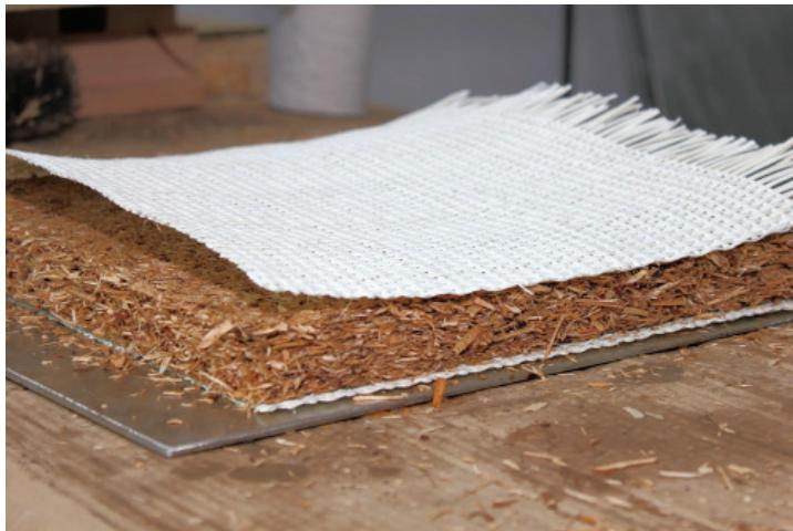
**Fig. 1. The mat after cold pre-pressing, covered by rattan mat**
