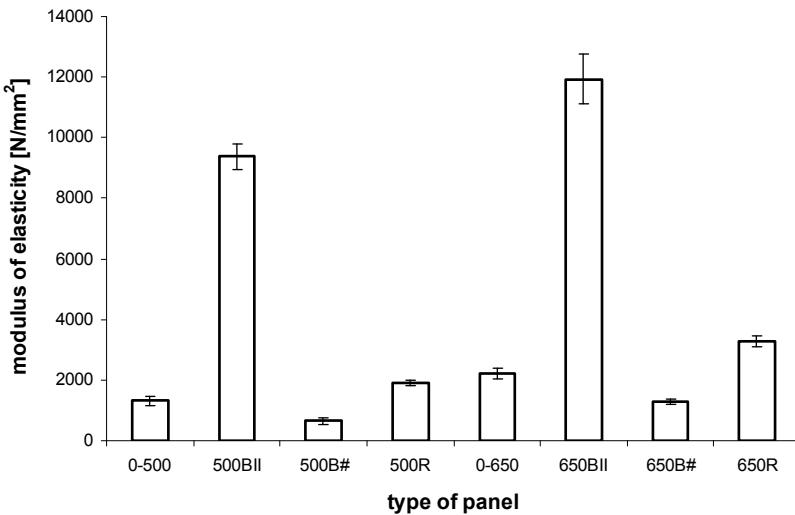
**Fig. 3. The values of modulus of elasticity of investigated panels**
