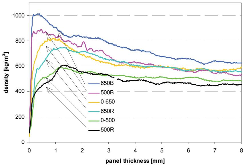
**Fig. 2.** The density profiles of the investigated panels (half thickness displayed)
