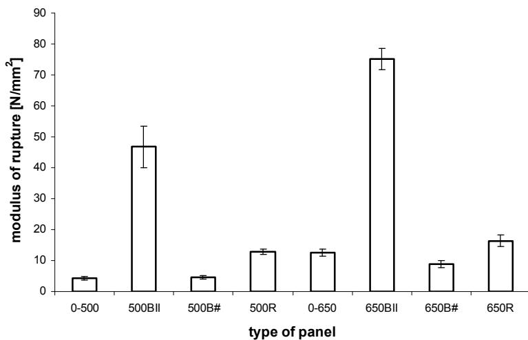
Fig. 4. The modulus of rupture of investigated panels
