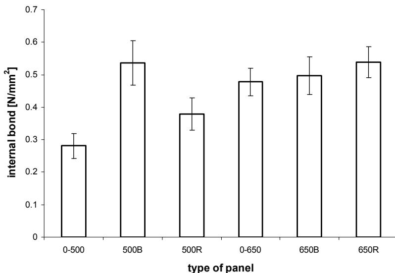
**Fig. 7. The internal bond of panels with surface layers made of fibrous materials**
