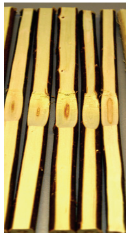
Fig. 1. The samples to measure the tensile strength of raw materials for fibrous chips production: assumed shape (a) and samples before test (b)
