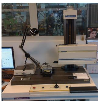
Fig.3. Profilographmeter FormTalysurf 120L
