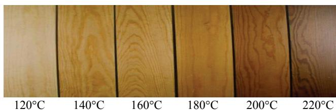
*Fig. 1. Change of coloration of pine wood during thermo-modification in different temperatures [5]*
