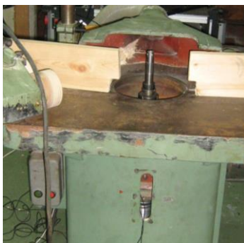
Fig.1. Universal wood shaper with bottom location of the working shaft
