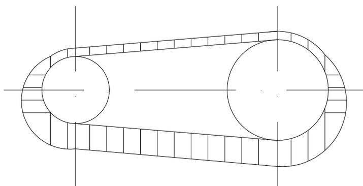
**Fig. 1.2 Belt loaded by working stroke**
