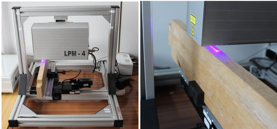
Fig. 5 For experimental measuring was used Laser profilometer LPM – 4
