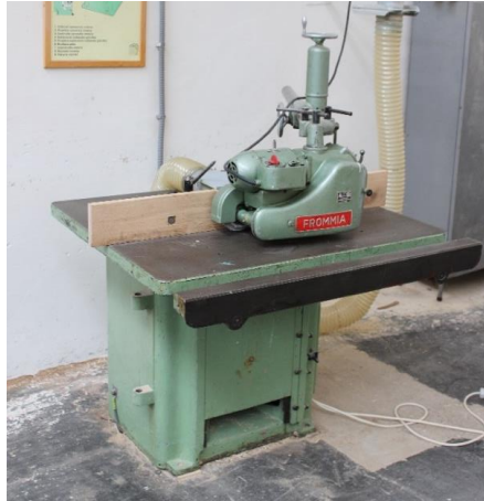
Fig. 2 Lower Spindle Milling Machine with attached Feeder
