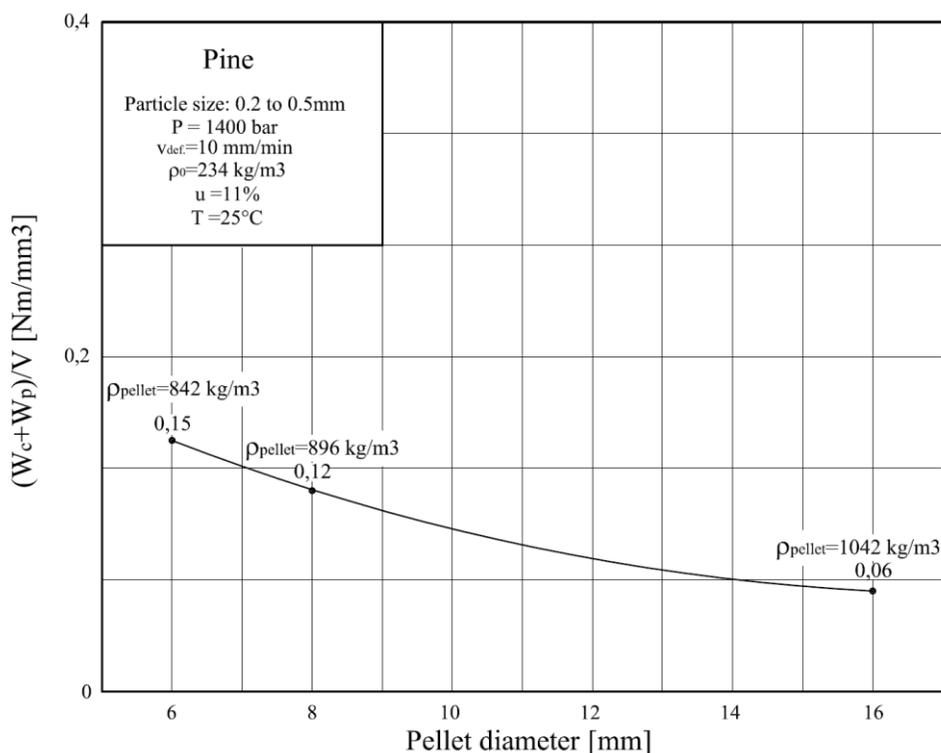
Figure 3. The change in specific work depending on the diameter of pine pellets at ambient temperature
