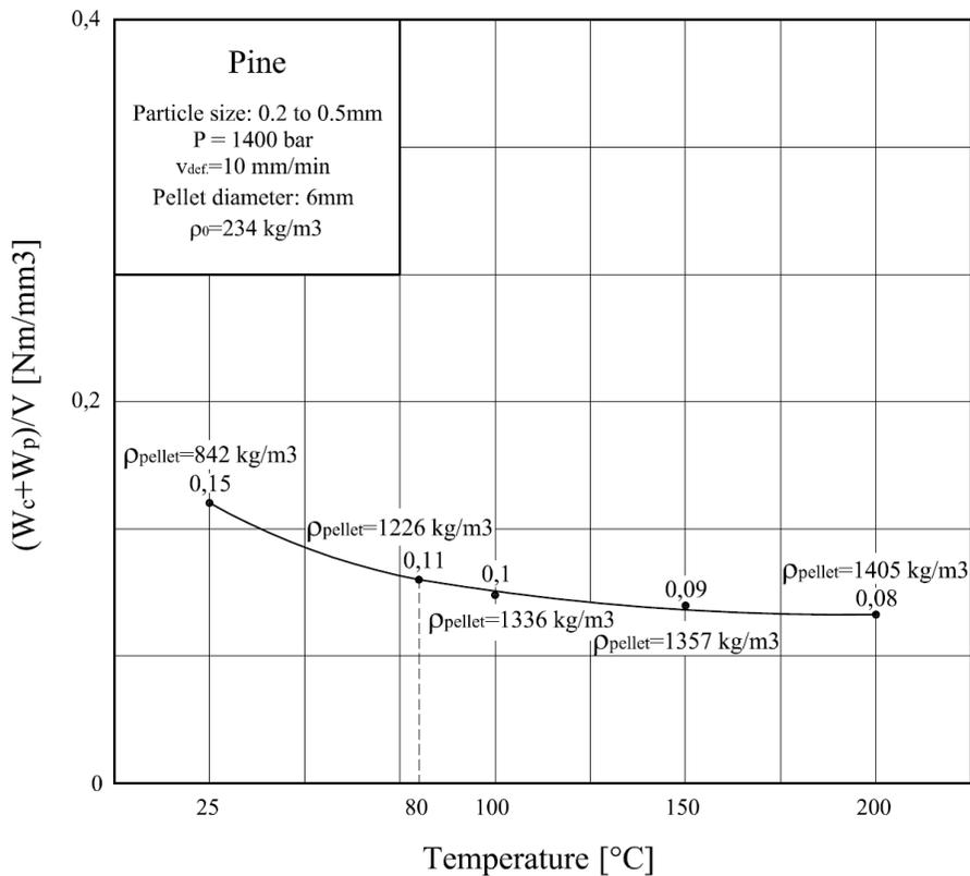
Figure 4. The change of total specific work depending on pellet temperature using pine chips
