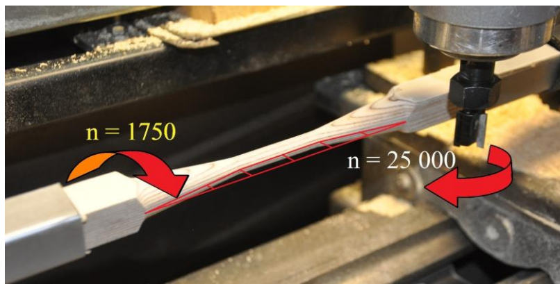
Fig. 4. Clamping of the sample in the lathe and the kinematics of the process
