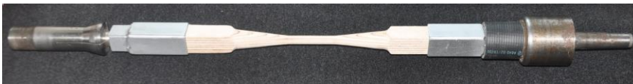
Fig. 3. Sample clamping in the grips and in the bushing and the tail centre
