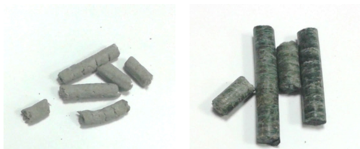
Fig. 4 Pellets from paper sludge with moisture content to about 51% (left) and 12% (right)
