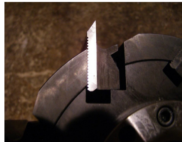
Figure 3 The milling head with hydraulic clamping with back fixation of planing blades
