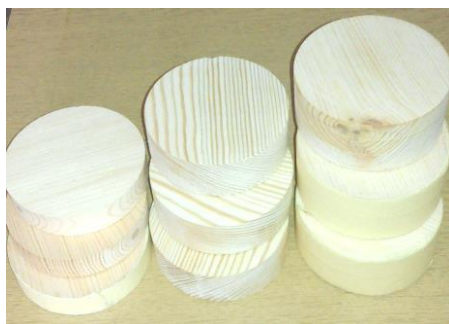
Figure 1. The tested specimens with different thickness
