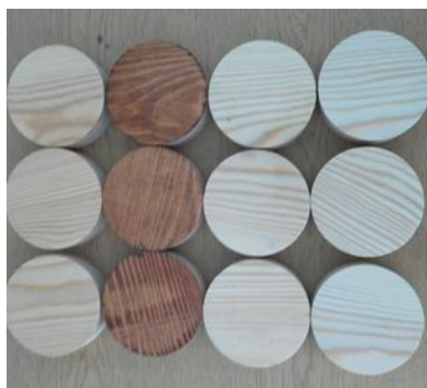
Figure 2. Specimens with different protective coatings
