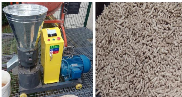
Fig. 1 Domestic device for pelletizing and sample A
