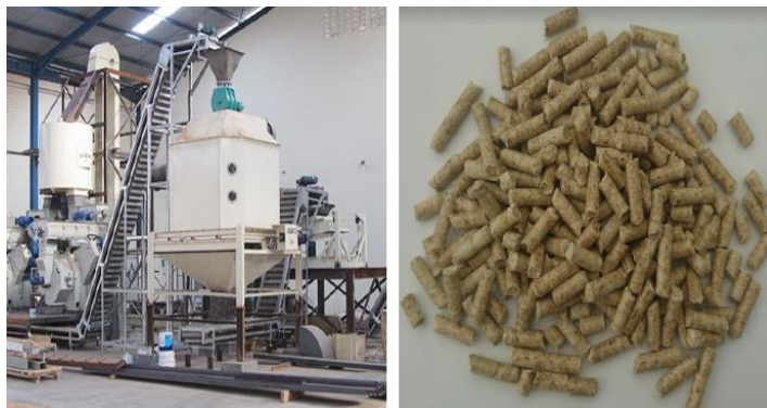
Fig. 2 Factory device for pelletizing and sample B
