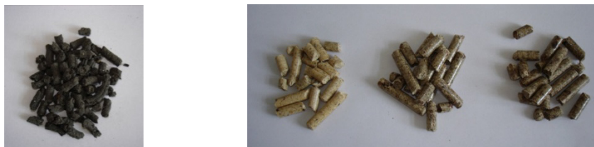
Fig. 2: Pellets of sewage sludge, clean sawdust spruce with an admixture of spruce bark
