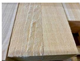
Fig. 1 Woolly surface and normal surface of beech blanks
