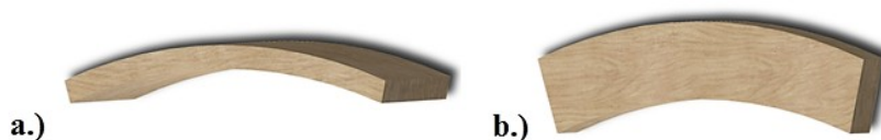
Fig. 3 Different types of longitudinal warping a.) bow b.) crook
