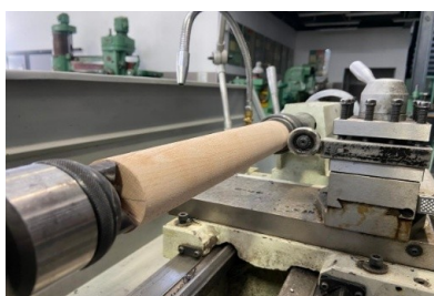
Figure 2. Densification of wood with the help of spinning roller.
