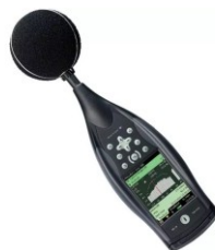
Figure 2 Measuring device with microphone and microphone cover
