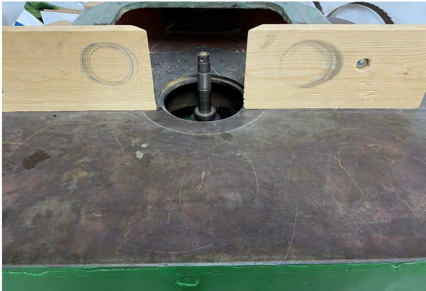
Fig 1. Wood shaper with bottom position of the spindle
