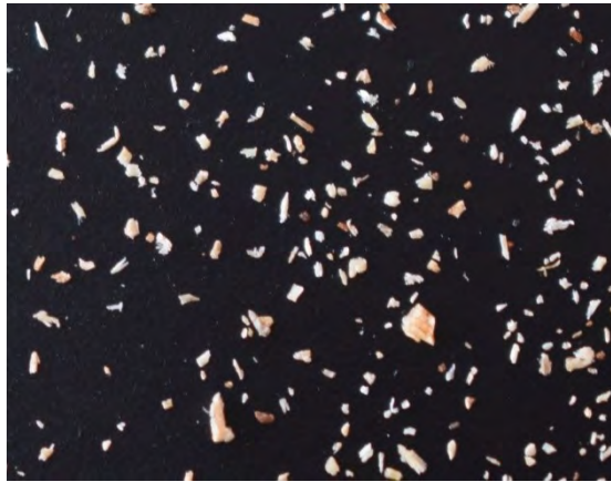
Figure 1 Obtained sawdust placed on a black contrasting base
