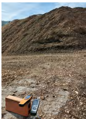
Fig. 1 Placement of the measurement point for dust meters
