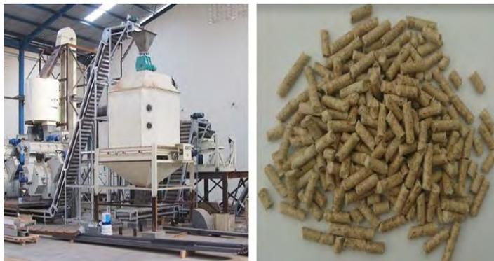
Fig. 2 Factory device for pelletizing and sample B
