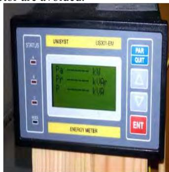
Figure 4. Measuring device, model *US301EM* – *Unisyst Engineering Ltd.*
