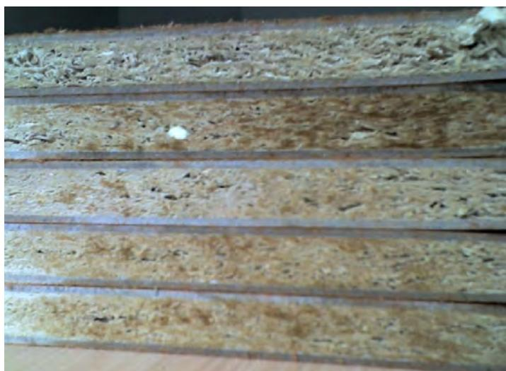
Ryc. 2. Double-sided coated of tested boards with hardboard.
