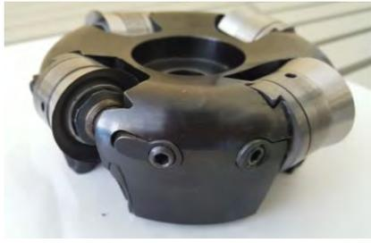
Fig.3. Standard milling head based on self-rotating blades
