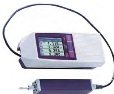
**Figure 2.** Profilometer, model Surftest SJ-210 – general view
