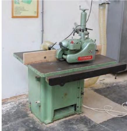
Fig. 2 Lower Spindle Milling Machine with attached Feeder
