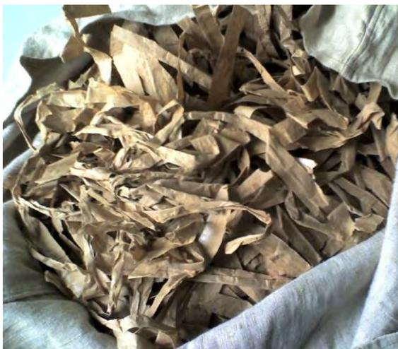
Ryc. 1. Paper strips coated on one side with polyethylene used in the research.
