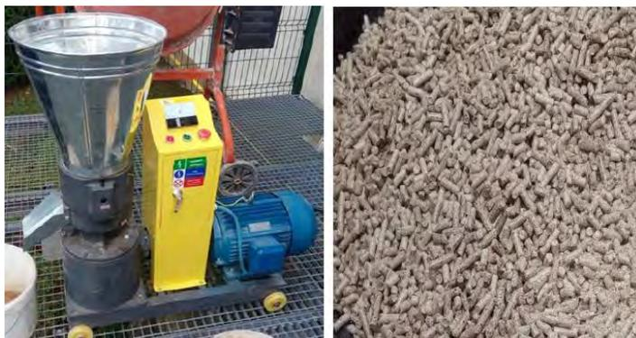
Fig. 1 Domestic device for pelletizing and sample A
