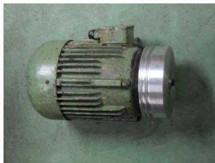
**Fig.2.** Electric motor with a pulley
