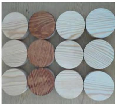
**Figure 2.** Specimens with different protective coatings
