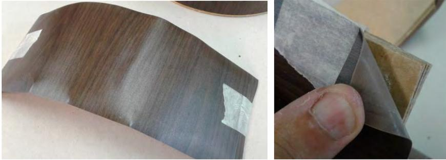
Figure 2. 1 - Test samples with poor adhesion between the PVC foil and the substrate;
