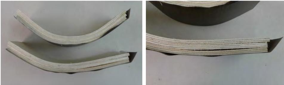
Figure 3. 1 - Self debonding of the test samples
