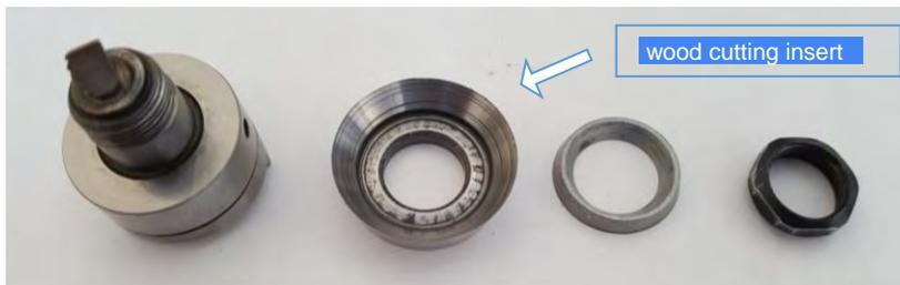
Fig.6. Construction of self-rotating SPRT tool blades
