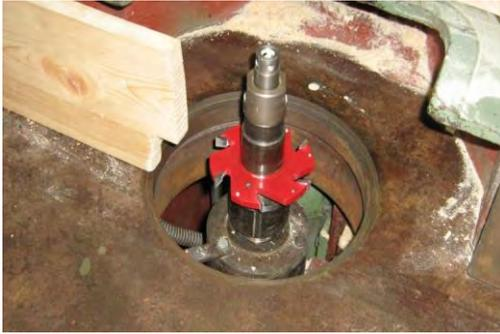
Fig.3. Groove cutter
