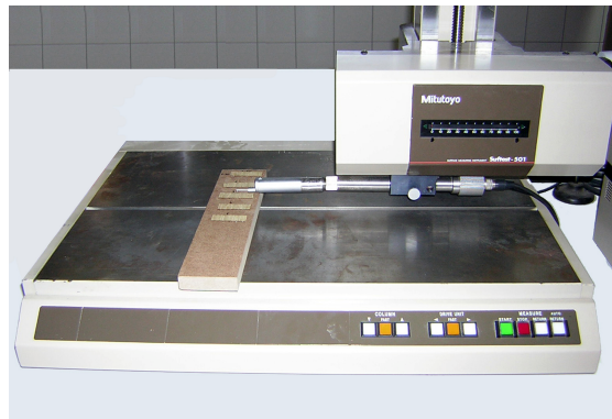
Fig 3 Surface quality tester "Surftest 501"
