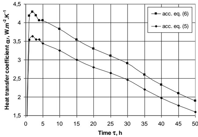
Fig. 3. Change in  $\alpha_r$  during 50 h freezing at  $t_{m1}^{fr} = -20$  °C of beech log with  $D = 0.24$  m,  $t_0 = 20$  °C, and  $u = 0.6$  kg·kg<sup>-1</sup>
