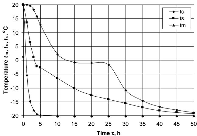
Fig. 2. Change in  $t_m$ ,  $t_s$ , and  $t_c$  of beech log with  $D = 0.24$  m,  $t_0 = 20$  °C, and  $u = 0.6$  kg·kg<sup>-1</sup> during 50 h freezing at  $t_{ml}^{fr} = -20$  °C
