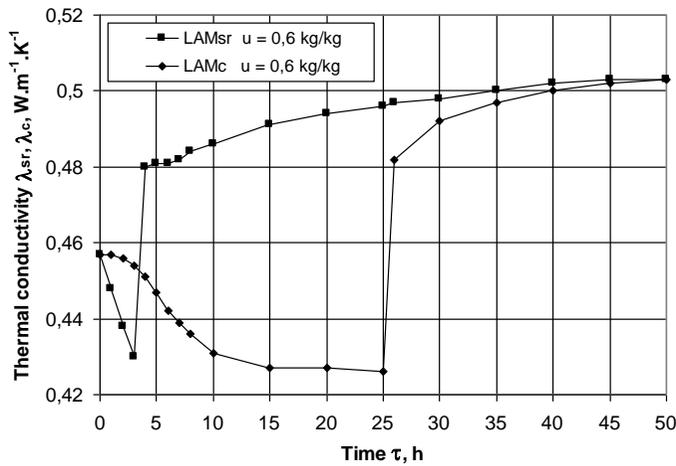
Fig. 4. Change in  $\lambda_{sr}$  and  $\lambda_c$  during 50 h freezing at  $t_{m1}^{fr} = -20$  °C of beech log with  $D = 0.24$  m,  $t_0 = 20$  °C, and  $u = 0.6$  kg·kg<sup>-1</sup>
