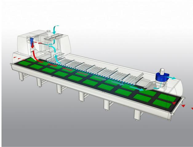
Figure 1. General view of equipment for unilateral convective heating of wood details before their subsequent lacquering
