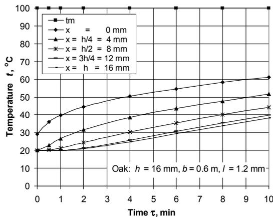
Figure 3. Change in  $t$  along the thickness of an oak detail with  $t_0 = 20^\circ\text{C}$ ,  $u = 0.08 \text{ kg}\cdot\text{kg}^{-1}$ , and  $l = 1.2 \text{ m}$  during its 10 min unilateral heating by air with  $t_m = t_{ha} = 100^\circ\text{C}$  and  $v = 5 \text{ m}\cdot\text{s}^{-1}$
