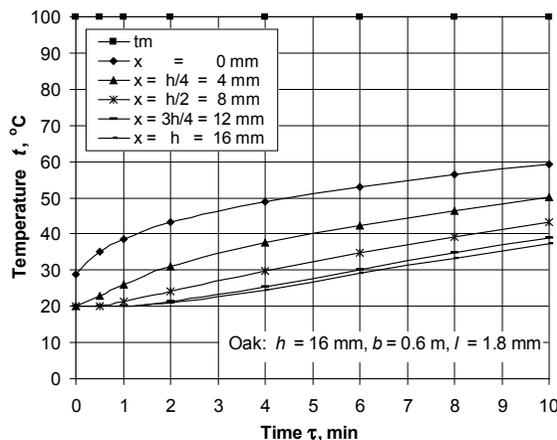
Figure 4. Change in  $t$  along the thickness of an oak detail with  $t_0 = 20^\circ\text{C}$ ,  $u = 0.08 \text{ kg}\cdot\text{kg}^{-1}$ , and  $l = 1.8 \text{ m}$  during its 10 min unilateral heating by air with  $t_m = t_{ha} = 100^\circ\text{C}$  and  $v = 5 \text{ m}\cdot\text{s}^{-1}$
