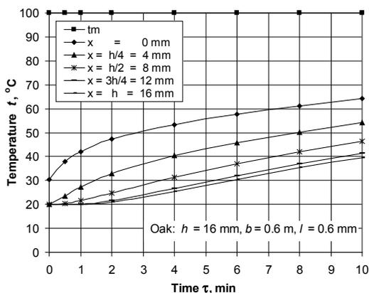
Figure 2. Change in  $t$  along the thickness of an oak detail with  $t_0 = 20$  °C,  $u = 0.08 \text{ kg} \cdot \text{kg}^{-1}$ , and  $l = 0.6 \text{ m}$  during its 10 min unilateral heating by air with  $t_m = t_{ha} = 100$  °C and  $v = 5 \text{ m} \cdot \text{s}^{-1}$
