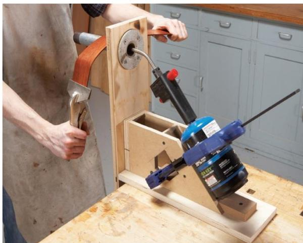
Figure 1. General view of equipment for bending of wood details used in the production of outside parts of the corpse of string music instruments
