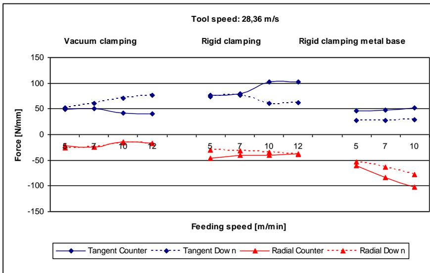
Fig 10. Tangential and radial forces in the capture of clamping varieties and feed speed.
