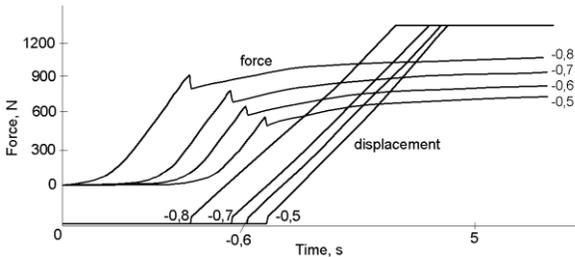
**Fig. 1. Force requirement for shifting of a workpiece on the machine table** (laminated particle board,  $A = 583 \text{ cm}^2$ , at different vacuum values)
