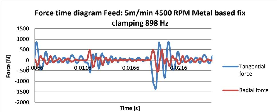
**Fig 11. The self-oscillation and the course of forces at rigid clamping**
