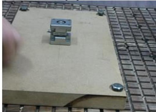
**Fig.7 Semi-rigid clamping screwed to an MDF sheet**
