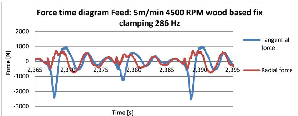
**Fig.12. The self-oscillation and the course of forces at semi-rigid clamping**
