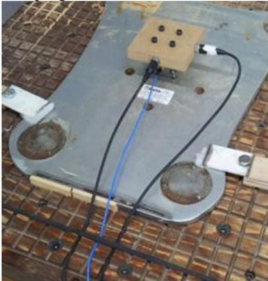
**Fig.6 Rigid clamping with steel plate**
