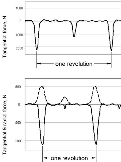
**Fig. 5 Unequal tooth feed and cutting force due to workpiece vibration clamped on a CNC-router and using a tool with two cutting edges. Upper Figure:  $n = 3,000$  rpm, feed speed 5 m/min, cutting depth 1 mm. Bottom Figure:  $n = 6,000$  rpm, feed speed 5 m/min, cutting depth 1 mm**
