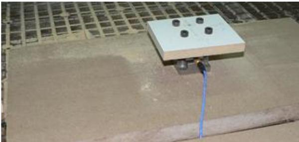
**Fig.8 Flexible vacuum clamping**
