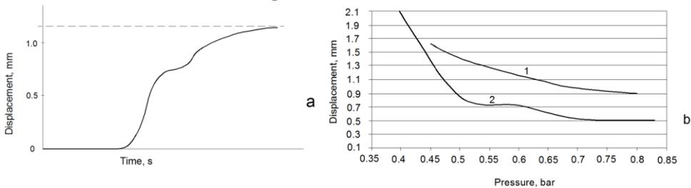
**Fig. 3 Displacement of an oak specimen under impact load (a); and displacement of oak (1) and chipboard (2) specimens as a function of clamping pressure (b). Impact mass 7.8 kg, drop height 7.5 cm, clamping vacuum 0.6 bar,  $A = 583 \text{ cm}^2$**
