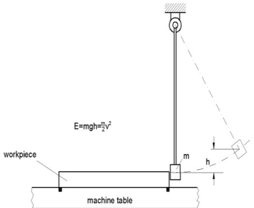
**Fig. 2. Pendulum loading device**
