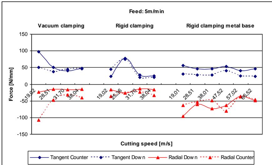
Fig 9. Tangential and radial forces in as a function of clamping varieties and cutting speed.
