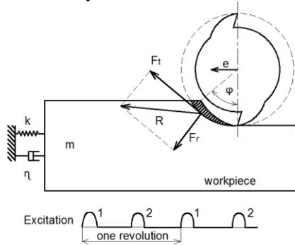
**Fig. 4 Excitation of a workpiece by periodic cutting forces**
