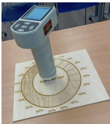
Figure 2. Colorimeter, model SC-30;
