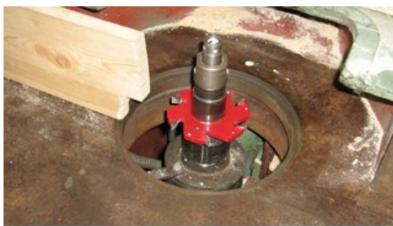
Figure 2. Groovecutter D=140 mm
