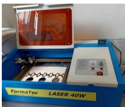
Figure 1. CO 2 laser machine for engraving and cutting
