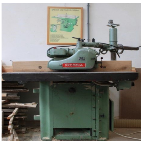
Fig. 3 Lower spindle milling machine FVS and feeder mechanism Frommia ZMD 252/137
