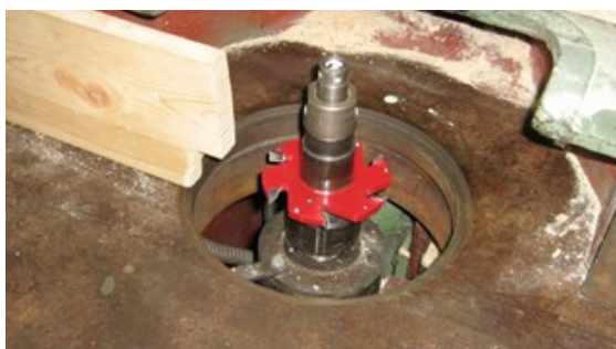
Figure 2. Groovecutter D=140 mm
