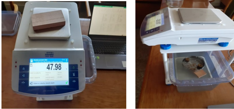
Fig. 1 Course of determination of wood density
