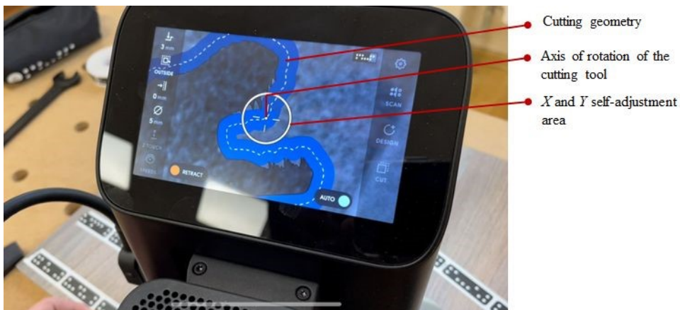
Figure 3. Software interface in cutting process (CNC Shaper Origin)
