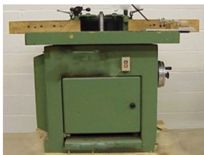
Figure 1. Wood shaper general view
