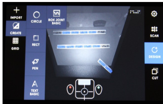
Figure 5. Software interface in design process (CNC Shaper Origin)
