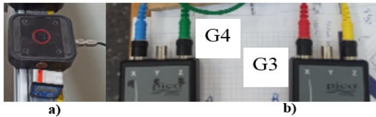
Fig. 1 a) pneumatic gripper with accelerometer b) color coding of measured axes
