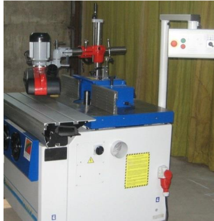
Figure 1. Woodworking spindle moulder machine, type T1002S with feeder
