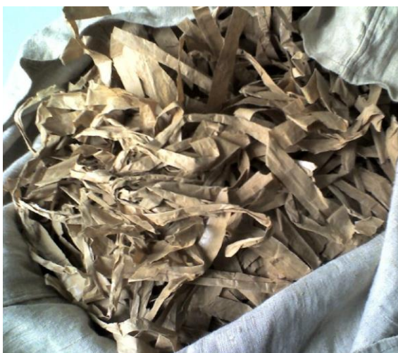
Ryc. 1. Paper strips coated on one side with polyethylene used in the research.
