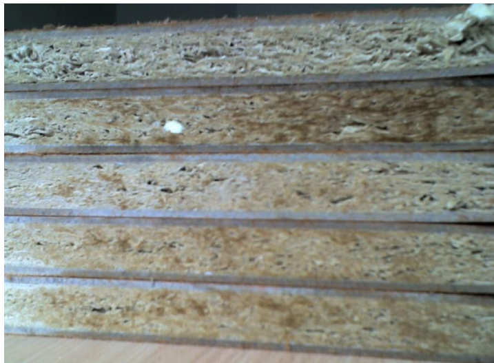
Ryc. 2. Double-sided coated of tested boards with hardboard.
