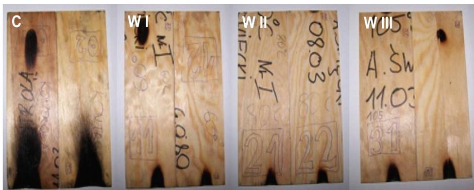
Figure 1. The condition of samples after the test for reaction to fire.
